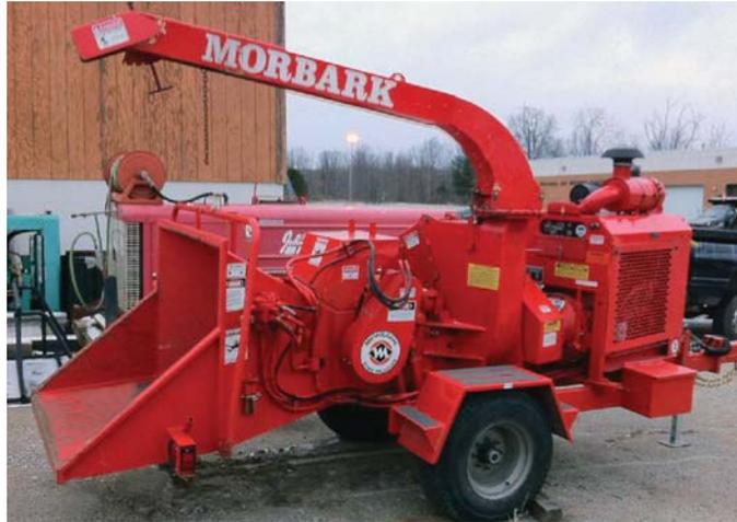
A wood chipper running on the University's own biodiesel prepares wood fuel for the boiler
